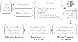
\*After the calibration is completed, the default operation mode is forward and reverse with brake function.
